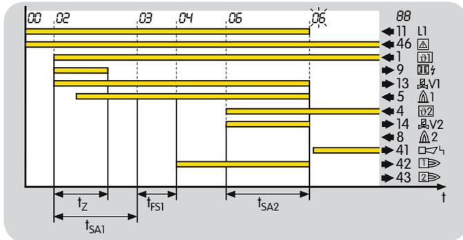
If no flame is formed during the start-up so that at the end of the safety time  $t_{SA1}$  no flame signal is detected, this will result in a BCU safety shut-down with subsequent fault lock-out. The fault message 05 will flash in the BCU display depending on the burner operating mode.
