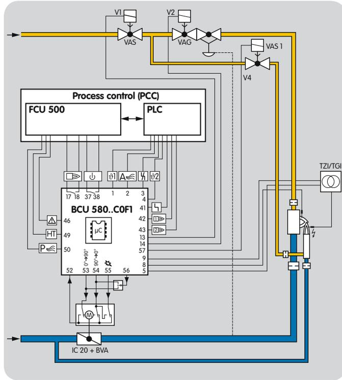
The BCU..F1/F2 activates a control element via the outputs for capacity control (terminals 53 to 56) for purging, cooling or starting the burner. This control element moves to the required position for the relevant operating situation.
