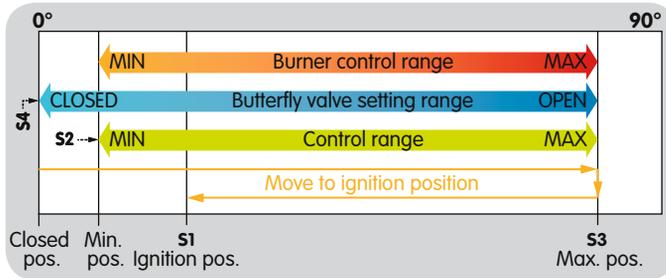
Parameter 75 = 3: IGNITION to MAX. capacity; standby in CLOSED position.
