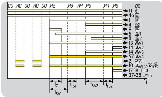
The air valve opens with the start-up fuel rate. The air valve can be activated externally via the input at terminal 2 for cooling the burner in the start-up position/standby.
