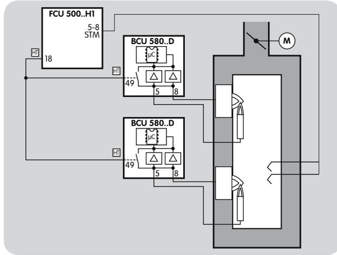
flame signals are once again monitored by a UV sensor or ionization electrode.
