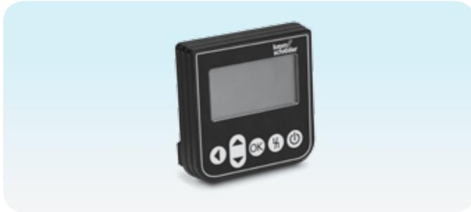
The OCU is an external operator-control unit which can be connected to a control unit of the FCU 500/BCU 500 series. The external operator-control unit OCU may be installed in the door of a control cabinet, for example. Thus, the control cabinet does not need to be opened to read out process values, statistics, flame signal intensities or parameter values, to change settings on the OCU or to control or adjust connected butterfly valves in Manual mode.
