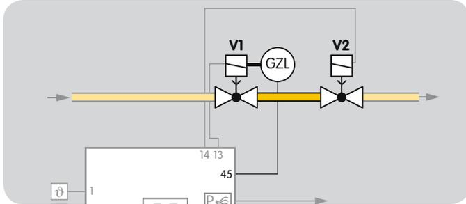
By checking the closed position using the proof of closure function, the BCU complies with the requirements of NFPA 85 (Boiler and Combustion Systems Hazards Code) and NFPA 86 (Standard for Ovens and Furnaces).
