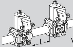
$$V_{p1} = V_V + L \times V_R$$
