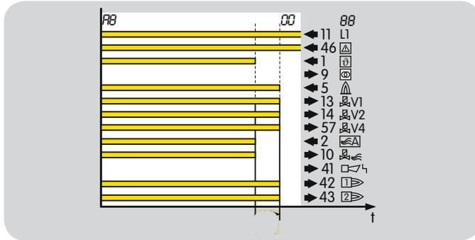
Parameter 43 = 0: Off. No low fire over-run is performed. The gas circuit is closed immediately owing to a quick closing gas valve in the case of On/Off control. The air circuit is closed more slowly. The air flowing in during this time increases the  $O_2$  content in the combustion chamber.
