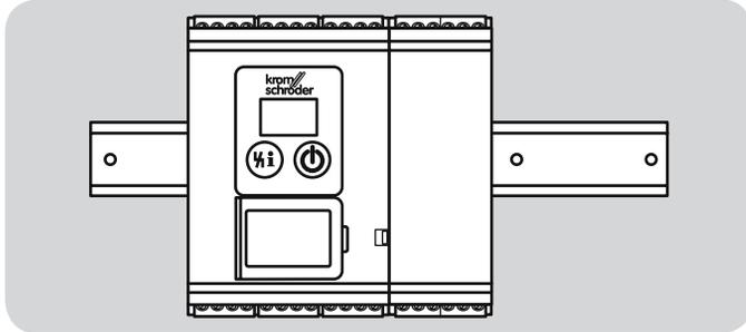
If the DIN rail is aligned vertically, end clamps are required (e.g. Clipfix 35 by Phoenix Contact) to prevent the BCU from slipping.
