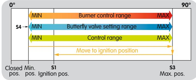
The minimum position which can be reached is the closed position.
