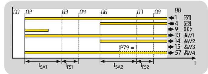
If a burner with a pilot burner is used, this parameter can be used to define whether the pilot burner is shut down 1 second before the end of the second safety time  $t_{SA2}$  or operates continuously.
