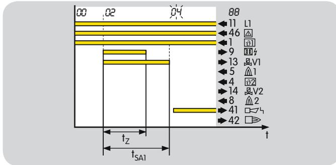
If no flame is formed during the start-up so that at the end of the safety time  $t_{SA1}$  no flame signal is detected, this will result in a BCU safety shut-down with subsequent fault lock-out. The fault message 44 will flash in the BCU display depending on the burner operating mode.
