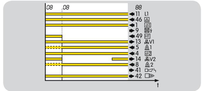
Despite the HT input having been disconnected from the electrical power supply, the burner remains in operation. The BCU performs flame control again (recommended in the case of ionization control or UV control with UVD).
