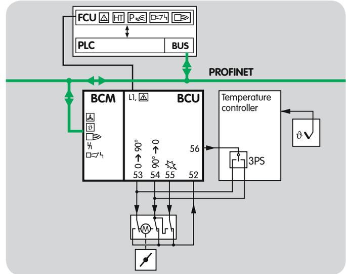
All network components which connect the automation system and the field devices must be certified for Profinet use.
