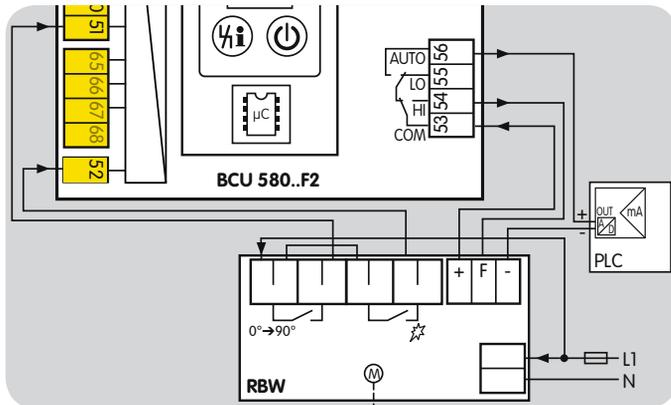
The RBW actuator reports that it has reached the position for maximum capacity via a signal to terminal 51. The actuator
