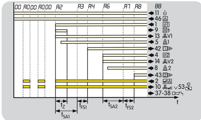
The air actuator can be activated externally via the input at terminal 2 during start-up. Parameter 48 must be set to 0 for this purpose, see also page 80 (Air actuator control).
