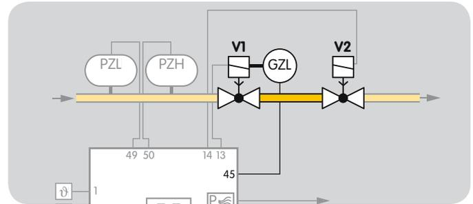
A signal is sent to the BCU via the POC switch on the gas solenoid valve on the inlet side before burner start-up stating that the valve is closed. After burner start-up, the signal must drop out to indicate to the BCU that the valve is open.
