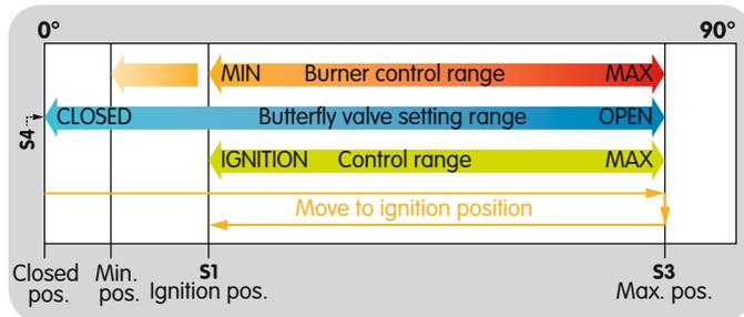
Parameter 75 = 4: MIN. to MAX. capacity; standby in position for MIN. capacity; burner quick start.
