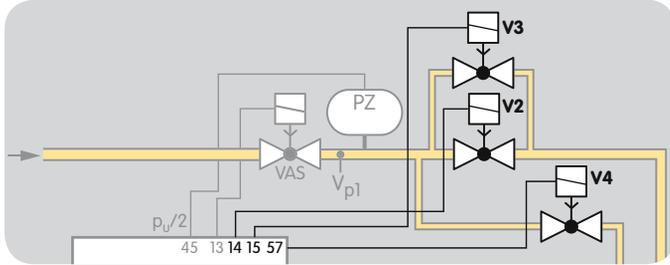
Parameter 52 = 2: V2. The test volume is discharged via the valve connected to terminal 14.
