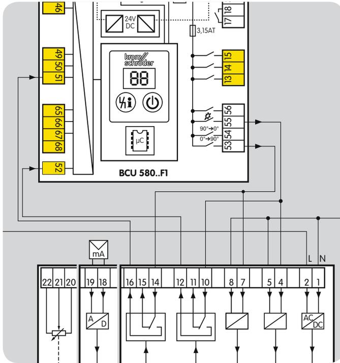
The positions for maximum capacity and ignition capacity can be set using the actuator. Terminal 51 checks whether the position for maximum capacity has been reached. Terminal 52 checks the position for ignition capacity. If the position is not reached within the timeout time of 255 s, a safety shut-down
