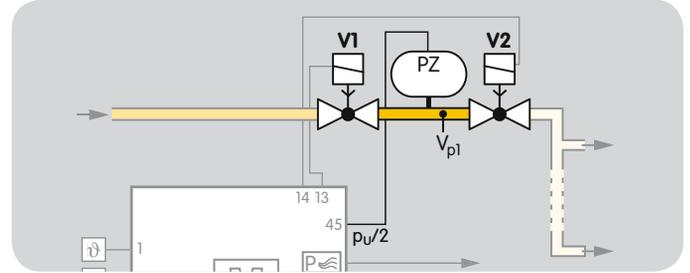
The required measurement time for the tightness test of  $V_{p1}$  can be set using parameter 56. The possible settings are 3 s, 5 to 25 s (in 5 s steps) or 30 to 3600 s (in 10 s steps).
