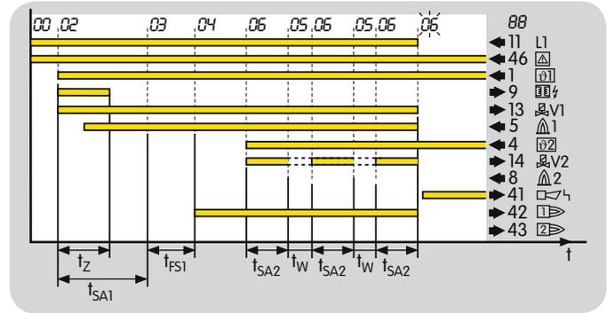
If no flame is formed during the start-up so that at the end of the safety time  $t_{SA2}$  no flame signal is detected, the BCU closes the gas valves and repeats the start-up. Each start-up attempt begins with the parameterized start-up behaviour.
