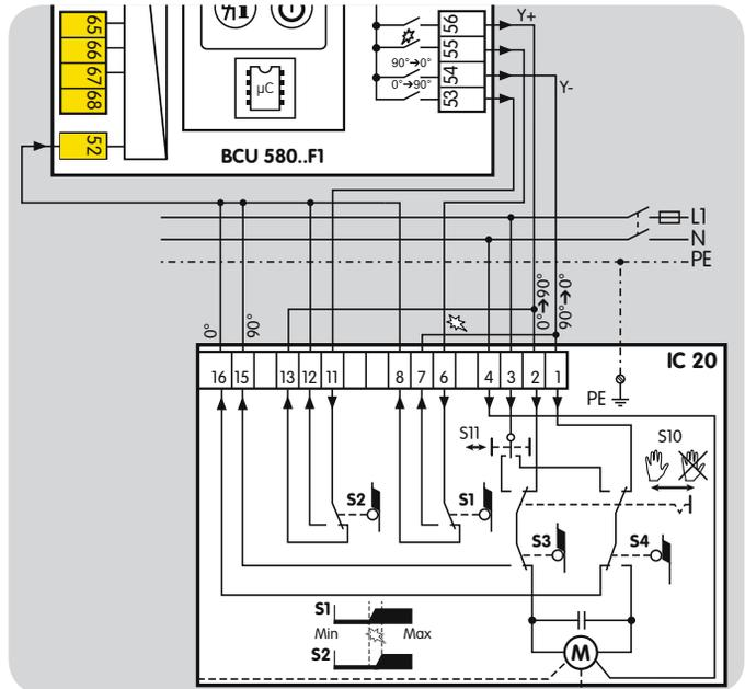
Parameter 75 = 5: IGNITION to MAX. capacity; standby in CLOSED position; burner quick start.
