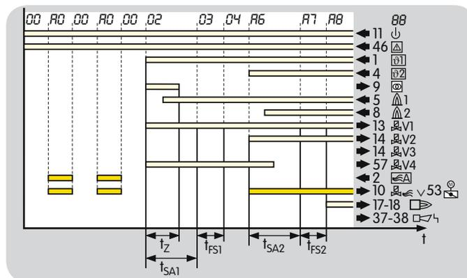
The air actuator opens at the same time as safety time  $t_{SA2}$  begins and the main burner starts.
