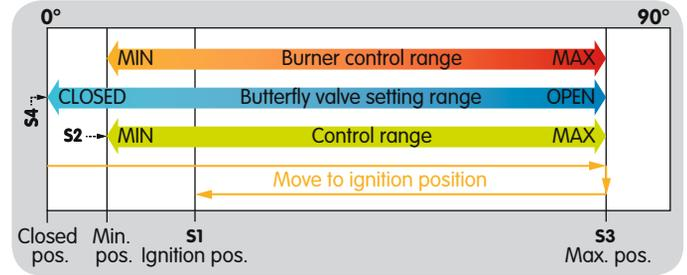
The control system is enabled for operation via the controller enable output (terminal 56). During the controller enable procedure, the actuator can be adjusted infinitely between the positions for maximum and minimum capacity by an external three-point step controller or using bus signals. There is no timeout active in this case.
