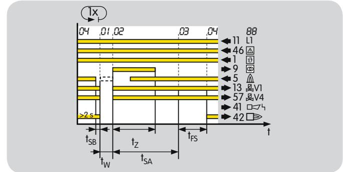
If a flame failure occurs during operation (minimum operating time of 2 s), the valves are closed and the operation signalling contact is opened within the safety time during operation  $t_{SB}$ . The burner control unit then attempts to restart the burner once. If the burner does not function, a safety shut-down with fault lock-out occurs. The display blinks and shows the fault message.
