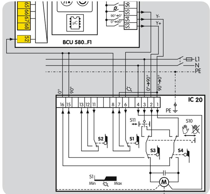
Parameter 75 = 2: MIN. to MAX. capacity; standby in CLOSED position. The control range while the burner is operating is between the positions for minimum capacity (S2) and maximum capacity (S3). The burner is ignited in the position for ignition capacity (S1). When the burner is switched off, the actuator is moved to the closed position (S4).
