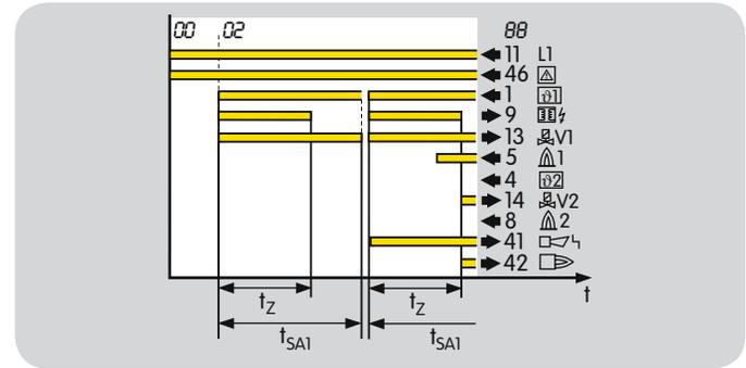
If no flame is formed during the start-up so that at the end of the safety time  $t_{SA1}$  no flame signal is detected, the BCU closes the gas valves and repeats the start-up. Each start-up attempt begins with the parameterized start-up behaviour.
