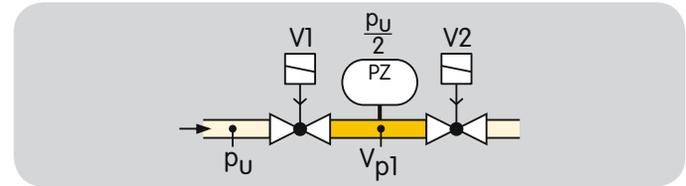
European standards EN 746-2 and EN 676 stipulate tightness controls for capacities over 1200 kW (NFPA 86: from 117 kW or 400,000 Btu/h).
