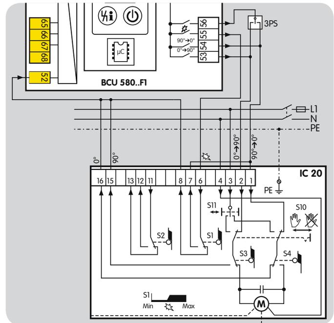
The positions for maximum capacity, ignition capacity and minimum capacity can be set using the actuator. It is checked whether the relevant position has been reached using terminal 52. If the position is not reached within the timeout time of 255 s, the BCU will display fault message  $R_C$ ,  $R_D$  or  $A_i$  (maximum, ignition or minimum capacity not reached), see page 47 (Fault signalling).
