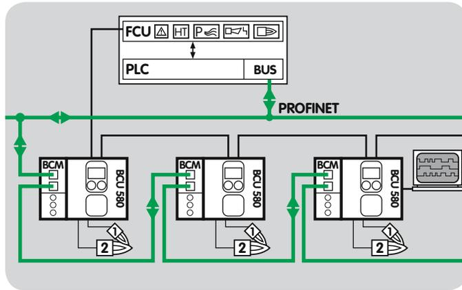
The bus system transfers the control signals from the automation system (PLC) to the BCU/BCM for starting, resetting, controlling the air valve, purging the furnace or for cooling and heating during operation. In the opposite direction, it sends operating status, the level of the flame signal and the current program status.
