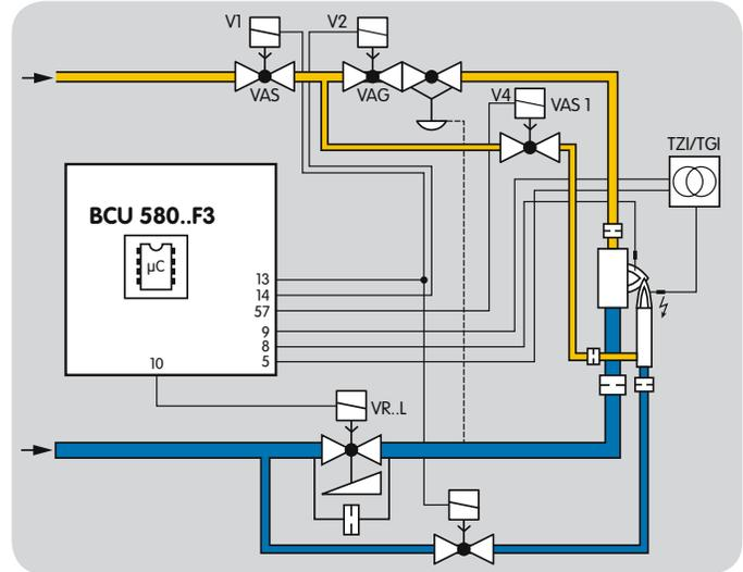
This means that the burner is initially adjusted down to low fire and then switched off completely. Flame control is still operational. It must be ensured that no excess gas occurs.
