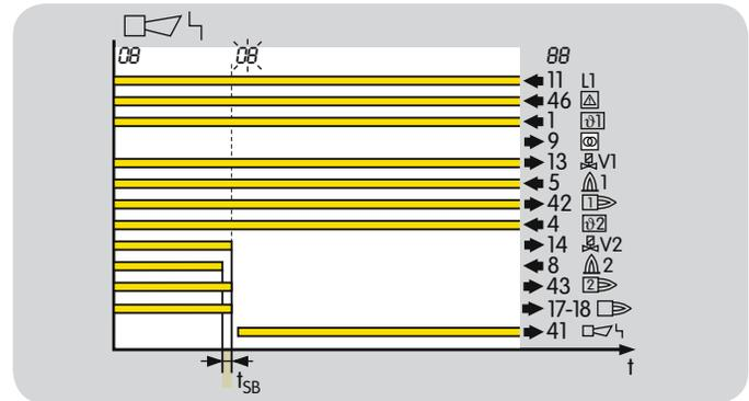
If the flame fails during operation, the output for valve V2 is disconnected within the safety time  $t_{SB}$ .
