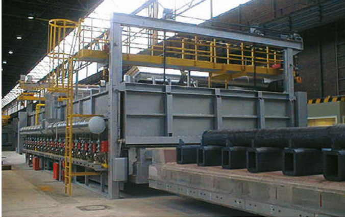
Metallurgical industry: bogie hearth furnace
