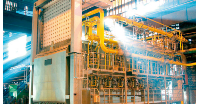
Ceramics industry: intermittent shuttle kiln
