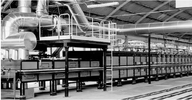
Roller hearth kiln in the ceramics industry
