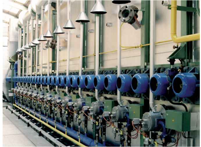
Roller hearth furnace
