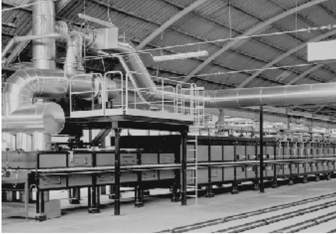
Roller hearth kiln in the ceramics industry
