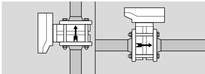
We recommend installing the butterfly valve in the vertical position with the direction of flow from bottom to top in order to prevent condensation and to prevent dirt from accumulating on the stop bar in the case of butterfly valves with stop bar.
