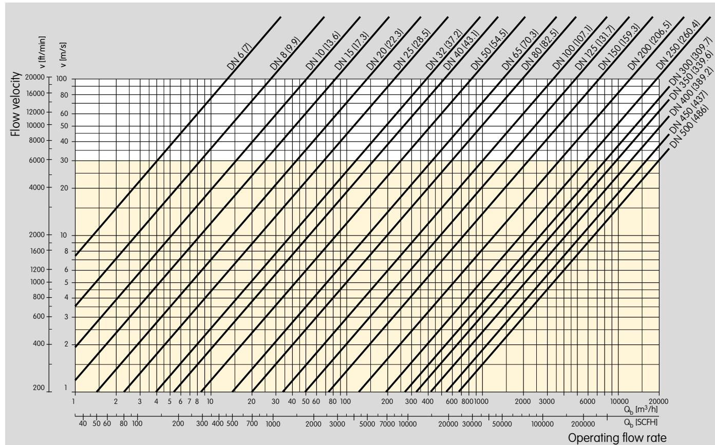
It is recommended that flow velocities of 30 m/s (5905 ft/min) are not exceeded when using the valve on thermoprocessing equipment.
