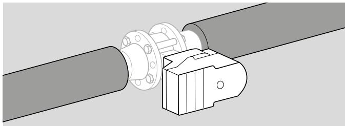
In conjunction with butterfly valves BVH, BVHS or BVHM for hot air, the actuators can be used in temperatures of up to 250°C (480°F), with additional heat deflectors they can be used in temperatures of up to 450°C (840°F).
